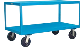
8" x 2" Phenolic casters Wheel brakes optional 34 1 / 4 " Overall height 4000 lbs capacity
