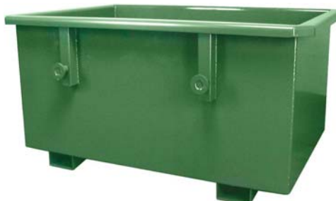
Extra heavy duty container fabricated from 3/8" plate. Designed for transport with overhead crane and to be emptied with rollover attachment on forklift. Used by bearing manufacturer.
